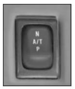
A power mode selector switch is included with the four-speed automatic transmission.
